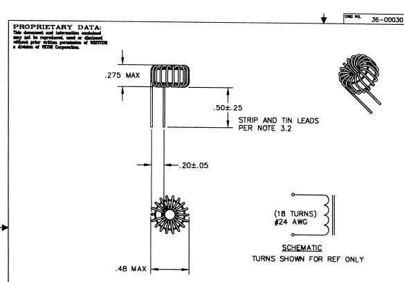
NOTE: CERTIFICATION OF MATERIAL COMPLIANCE REQUIRED. COMPLETED ASSEMBLY MUST BE (RoHS) COMPLIANT PER VICOR SPEC CST-0001.
